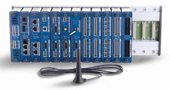
T-BOX MS combines the power of the Internet with modular-based architecture to create a class-leading remote control and automation solution. Equipped with one of the market's most powerful processors, only T-BOX incorporates Web server technology with SMS reporting and remote control to give you real-time access anytime, anywhere, using a standard Web browser.
